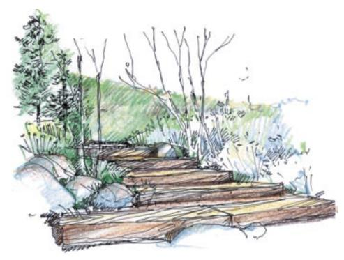
FIGURE 2-8: Wood steps with gravel treads blend into the wooded landscape
