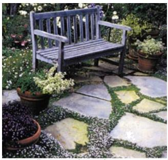
Spaced pavers allow water to percolate into soil
