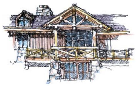
Balconies and decks are constructed of wood and detailed to match the building's architecture
