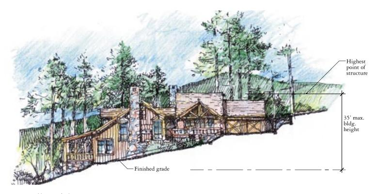
FIGURE 3-4: Building Height diagram
